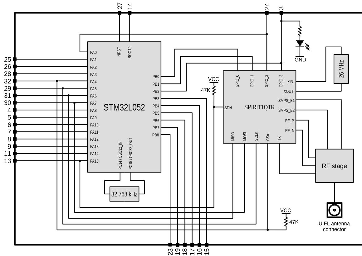
Figure 2 - Simplified schematic of XLN-RF-C module
