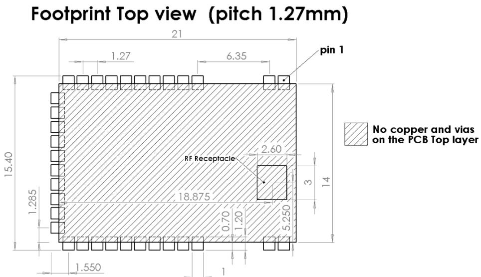
Figure 3 - Recommended PCB footprint
