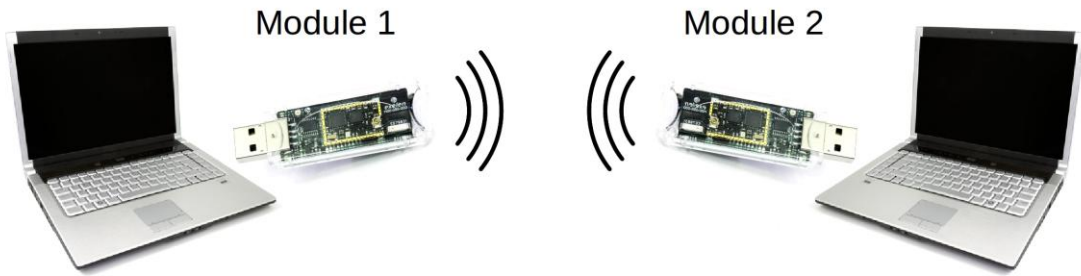
Figure 1 - Example setup with 2 PCs communicating wirelessly through XLN-RF-868-USB modules
